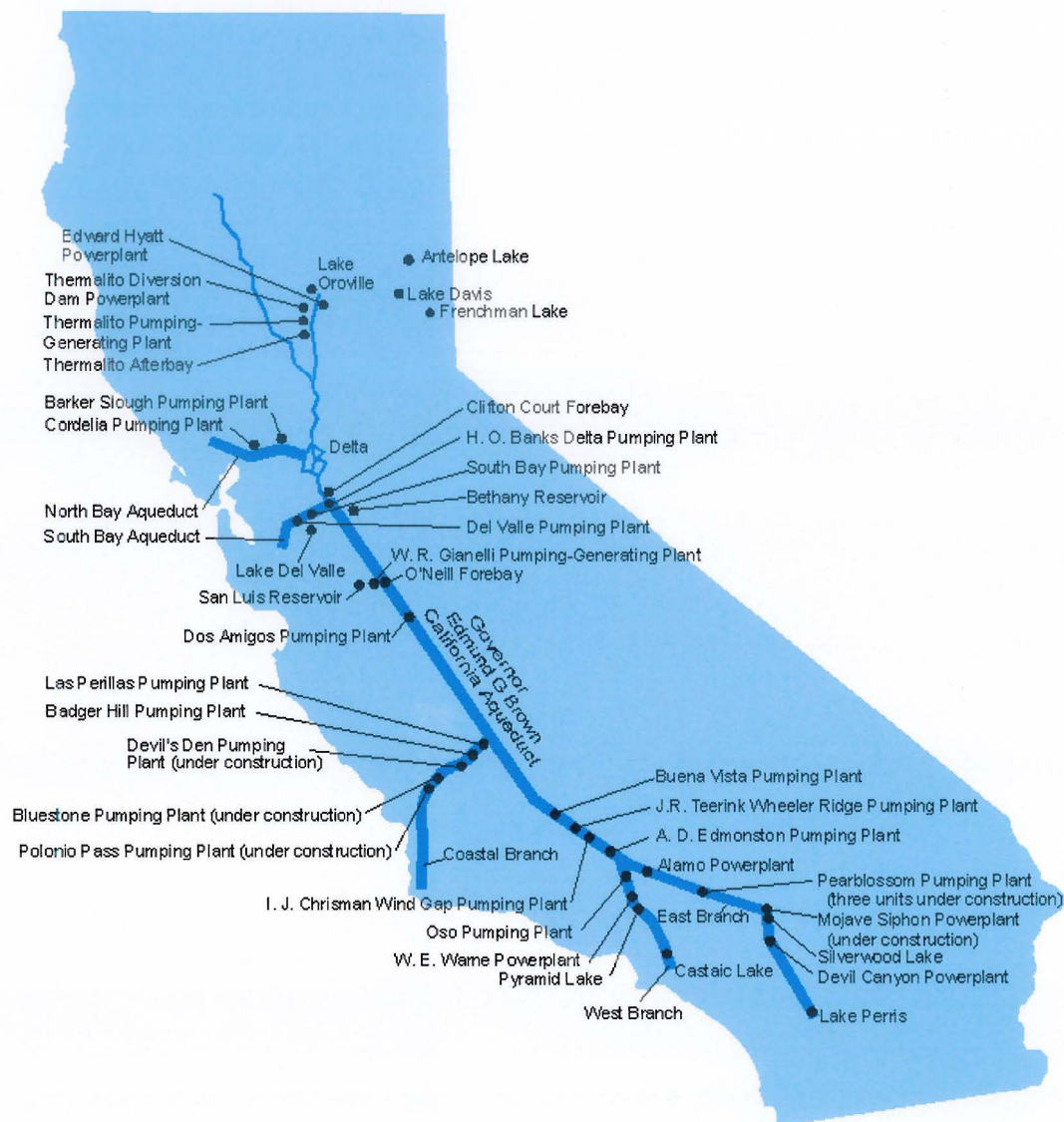
Figure 4. California State Water Project Facilities (CA SWP Website, 2011)
